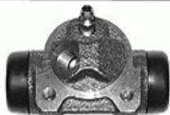
1. 673 177 links/left System: Bendix Ø 17,46 mm >1986
