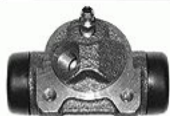
1. 673 177 links/left System: Bendix Ø 17,46 mm >1986 - 4x4
